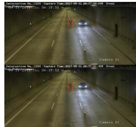
Pedestrian Detection Large area coverage / small target detection (48*48 pixels)
