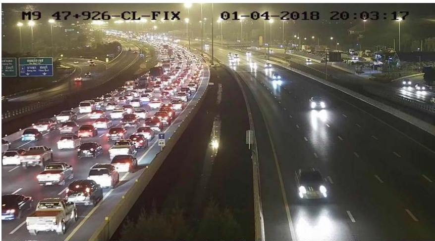
Congestion Detection 150m traffic jam recognition with adjustable detection sensitivity level. (48*48 pixels)
