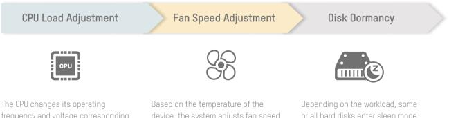
frequency and voltage corresponding to system load intelligence and lowers the power consumption without affecting operation. Based on the temperature of the device, the system adjusts fan speed – up to 20 levels of speed (about 1°C per level adjustment). Depending on the workload, some or all hard disks enter sleep mode, reducing power consumption and prolonging hard disk life.
